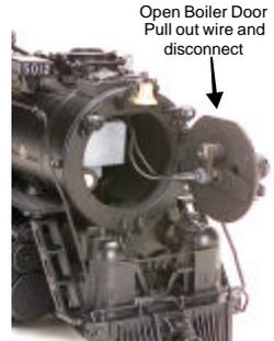
*Figure 8a. Replacing the Headlight*
