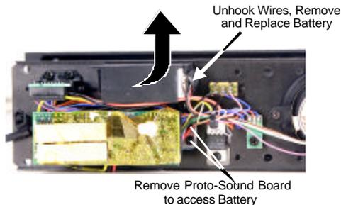
*Figure 11. Replacing the Battery*
