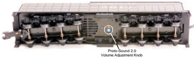
Figure 2. Manually Adjusting the Proto-Sound 2.0 Volume
