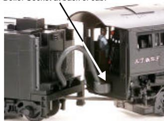
Figure 1a. Connect the Tender to the Engine
