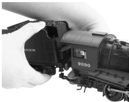
Figure: Connecting Locomotive to Tender
