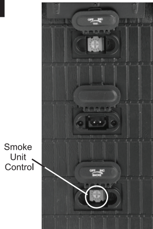
Figure 2: Smoke Unit Control Location
