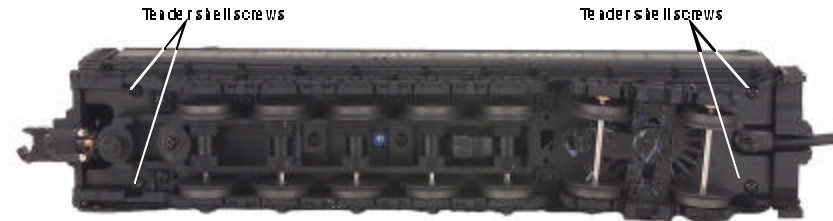
Figure 9. Screws to remove the tender shell
