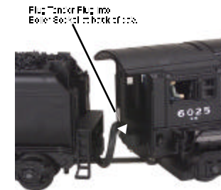
Figure 1a. Connect the Tender to the Engine
