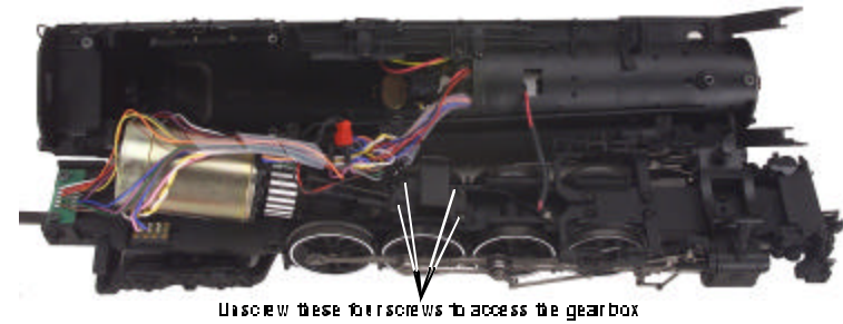
Figure 7b. Screws to remove to access the gear box.
