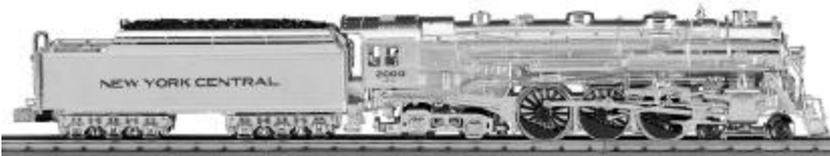
Thank you for purchasing the MTH Electric Trains die-cast J1e steam locomotive. This 1/4" scale reproduction of the famous J1e locomotive measures over 29" in length and weighs over 14 pounds. Despite its scale size, the locomotive is capable of operating on O-54 3-rail track and compatible AC transformers, (see page 33 for a complete list of compatible transformers and wiring instructions) and is completely compatible with most other 3-rail locomotives, rolling stock and accessories.
