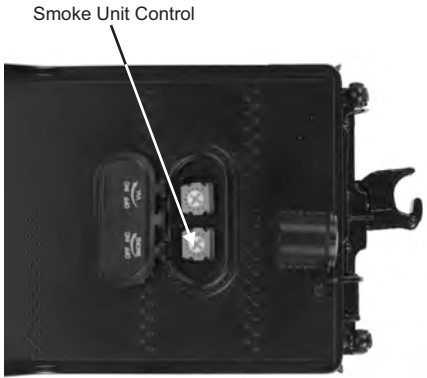
Figure: Smoke Unit Control
