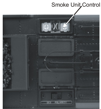
Smoke Unit Control Location
