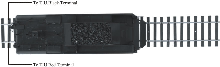
Proper 2-Rail polarity wiring and locomotive orientation
