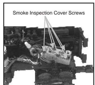
Figure 15: Smoke Unit Inspection Cover
