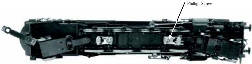
Figure 2: 3-Rail Pickups installed with a single Phillips Screw
