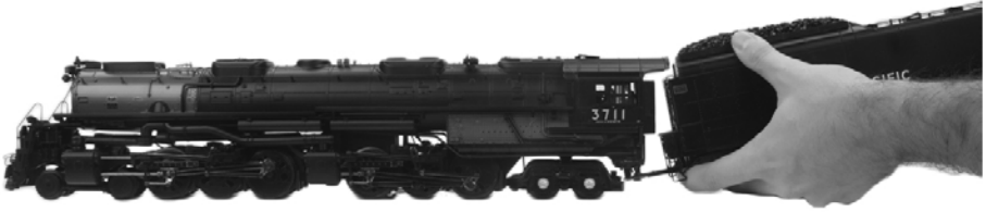
Figure 5: Connecting Locomotive to Tender
