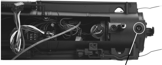
Remove Screw to access headlight
