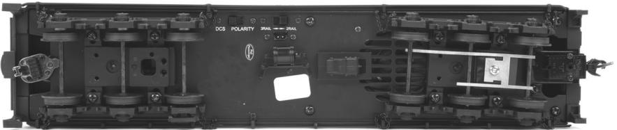
Kadee® Coupler Bracket Installed
