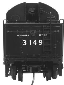
Kadee® Coupler Bracket Installed
