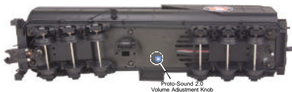
Figure 2. Manually Adjusting the Proto-Sound 2.0 Volume
