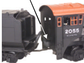
Figure 1a. Connect the Tender to the Engine
