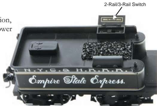
Figure 7: Selecting 2-rail or 3-rail power input setting
