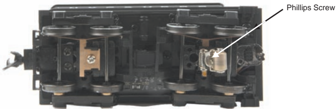
Figure 6: 3-Rail Pickups installed with a single Phillips Screw
