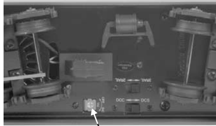
Proto-Sound® 3.0 Manual Volume Control
