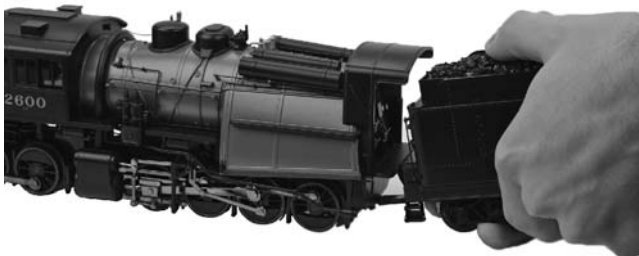
Figure 4: Connecting Locomotive to Tender
