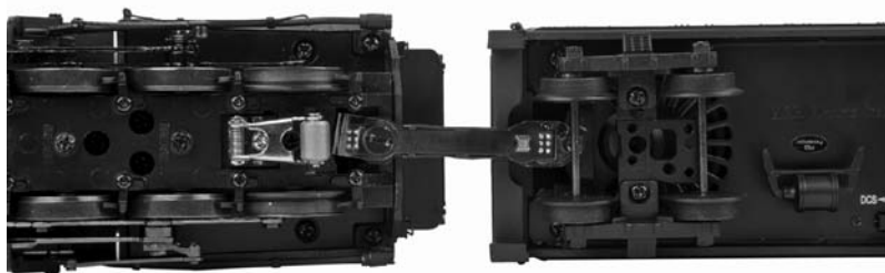
Figure 6: Correct connection of Engine and Tender
