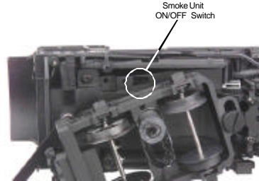
Figure 3: Smoke Unit Switch Location
