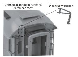
If you would like to install Kadee® Couplers on your cars, do not attach the diaphragm supports. This will allow less tension when the diaphragms touch each other. Kadee® Couplers cannot operate with this set when you have the supports on.
