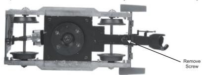
To remove the linkage you will need to remove the 4 truck side screws and remove the truck sides. After the truck sides are removed lower the truck frame and remove the linkage. Then reassemble the truck.
