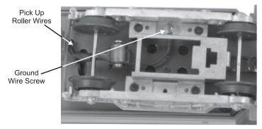
Next you will need to remove the small screw on top of the truck to free the coupler.
