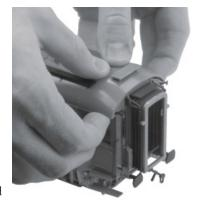
Once the roof is removed you will see the two light boards. Remove the 4 screws and lower the boards out. Replace with new light boards and reassemble in reverse order.
