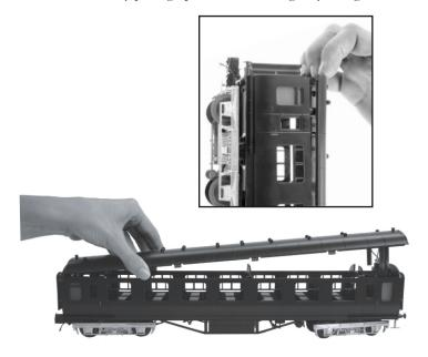
Once the body is removed you will see the two light boards. Remove the 4 screws and lower the boards out. Replace with new light boards and reassemble in reverse order.
