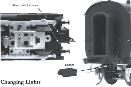
Occasionally, the lights inside the car may need to be replaced. To replace the lamps follow the disassembly instructions on the following illustrations. Replacement lamps can be obtained directly through MTH Electric Trains (Order online: www.mthtrains.com, e-mail: parts@mth-railking.com,Fax: 410-423-0009, Phone: 410-381-2580, Mail: 7020 Columbia
