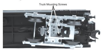
Then disconnect the wires from the pick-up roller and unscrew the ground wire to free the truck from the car.
