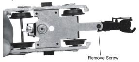
To remove the linkage you will need to remove the 4 truck side screws and remove the truck sides. After the truck sides are removed lower the truck frame and remove the linkage. Then reassemble the truck.
