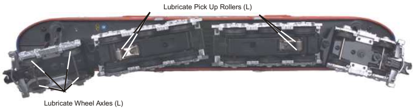
Figure 1. Lubrication Points on the Locomotive
