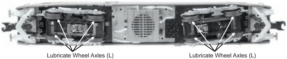
Figure 1. Lubrication Points on the Locomotive
