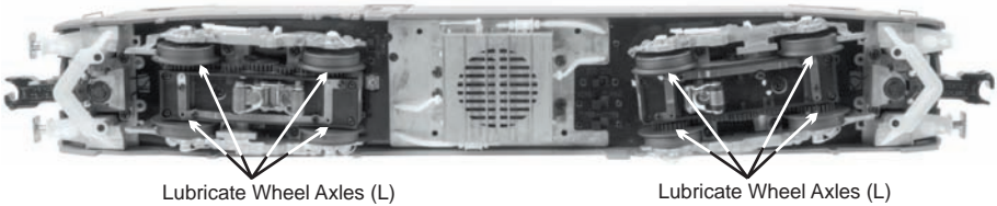
Figure 9: Lubrication Points on the Locomotive
