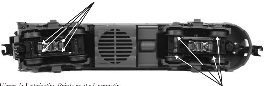
Figure 1: Lubrication Points on the Locomotive
