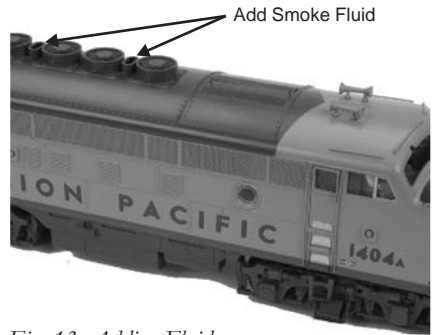
Fig. 13: Adding Fluid The smoke unit control potentiometer is located at the rear end of the Lead A unit
