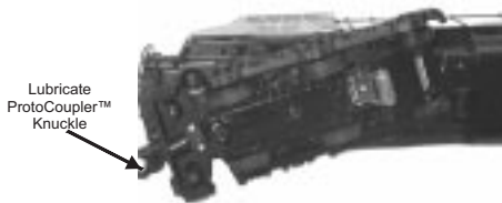
Figure 3: Lubricating The ProtoCouplers
