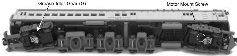
Figure 7. Locations of Greasing Points on the Locomotive
