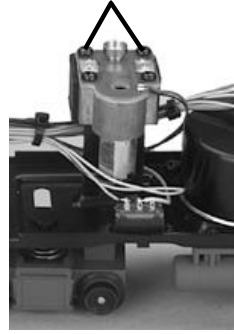
Figure 4. Inspecting the Smoke Unit
