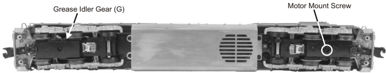
Figure 7. Locations of Greasing Points on the Locomotive
