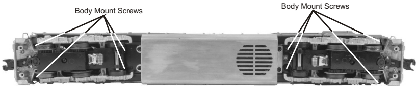
Figure 6. Locations of the Body Mounting Screws
