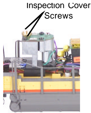
Figure 4. Inspecting the Smoke Unit
