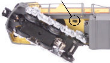
Figure 3. Smoke Unit ON/OFF Switch
