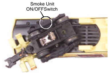
Figure 3. Smoke Unit ON/OFF Switch
