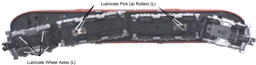
Figure 1. Lubrication Points on the Locomotive
