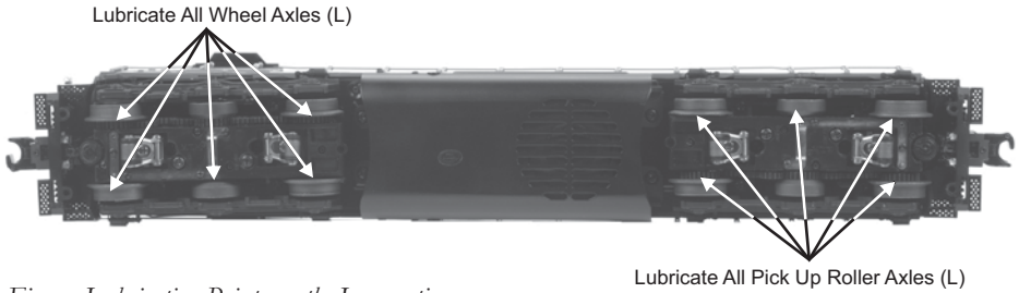
Figure: Lubrication Points on the Locomotive
