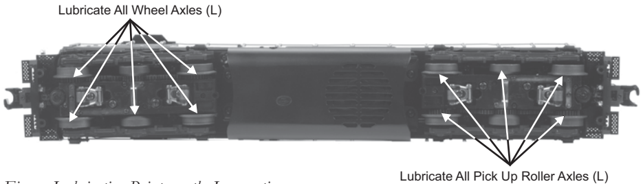
Figure: Lubrication Points on the Locomotive
