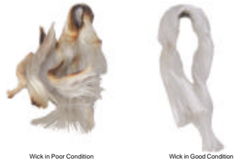
Figure 7. Examples of a wick in poor condition and in good condition.
