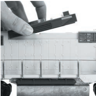
Lift Cover to access Smoke Unit
