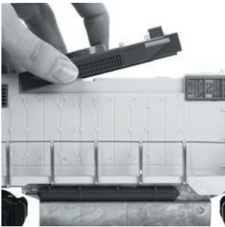
Lift Cover to access DCS Polarity Switch
