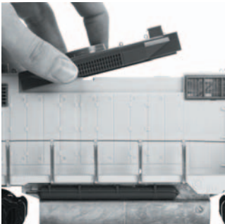
Lift Cover to access Smoke Unit
