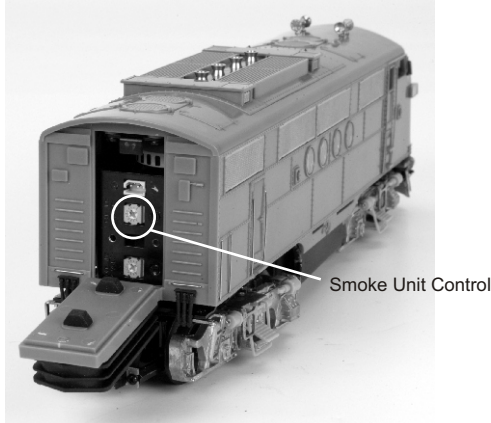
Smoke Unit Control
