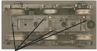
Remove (4) bottom plate mounting screws.
