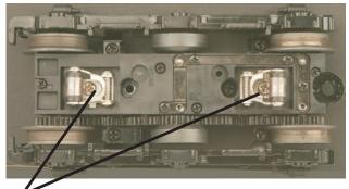
Remove pickup roller mounting screws.
