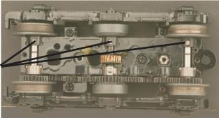
We *strongly* recommend replacing each wheel set on each truck, one at a time to prevent mixing up the wheel sets and truck blocks.
