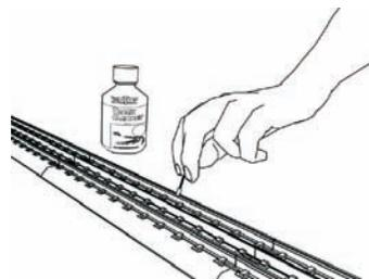
To clean the track, use RailKing Track Cleaning Fluid found in Maintenance Kit (30-50010) or denatured (not rubbing) alcohol and a clean rag. Unplug the transformer and wipe the rails of the track, turning the rag frequently to ensure that you are using clean cloth on the rails. Thereafter, keep an eye on the track and clean it when it gets dirty to ensure good electrical contact and to lengthen the life of the tires.
