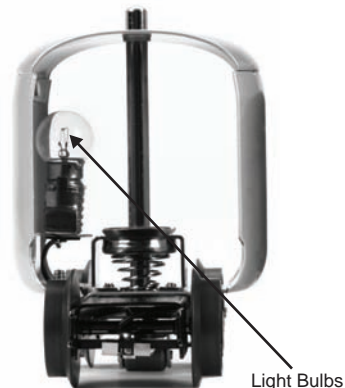
Figure 13: Vestibule Light Bulb
