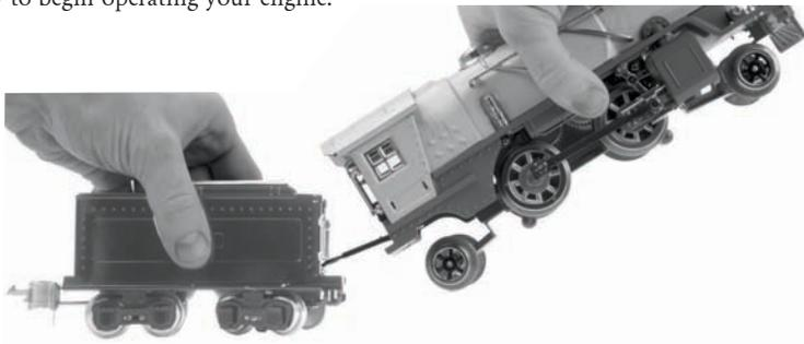
*Figure 5: Connecting Engine and Tender*
