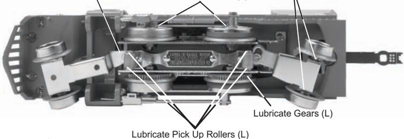
Lubricate Pick Up Rollers (L)
