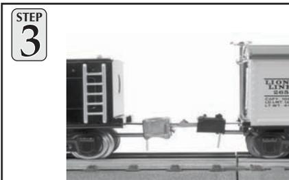
To couple passenger cars and tender together, you will have to manually align hooks and gently push box couplers together.
