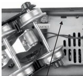
Figure 7: DCS/DCC Switch
