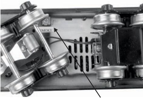
Figure 2: Smoke Unit Control (on bottom of tender)
