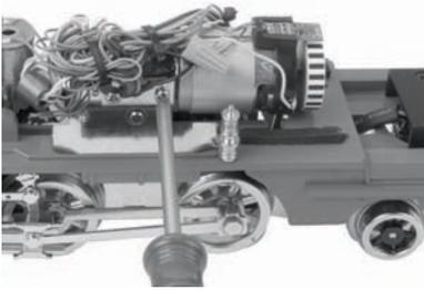
Fig. 12: Unscrewing Gearbox screws
