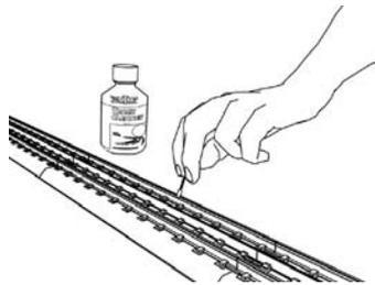
To clean the track, use RailKing Track Cleaning Fluid found in Maintenance Kit (30-50051) or denatured (not rubbing) alcohol and a clean rag. Unplug the transformer and wipe the rails of the track, turning the rag frequently to ensure that you are using clean cloth on the rails. Thereafter, keep an eye on the track and clean it when it gets dirty to ensure good electrical contact and to lengthen the life of the tires.
