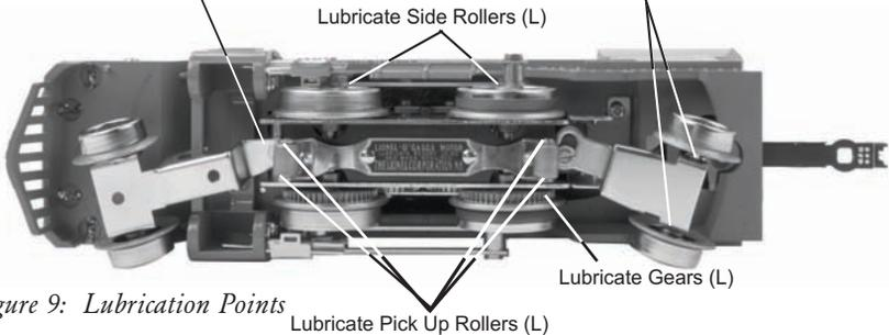
Figure 9: Lubrication Points
