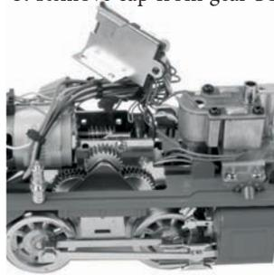
Fig. 13: Removing Cap
