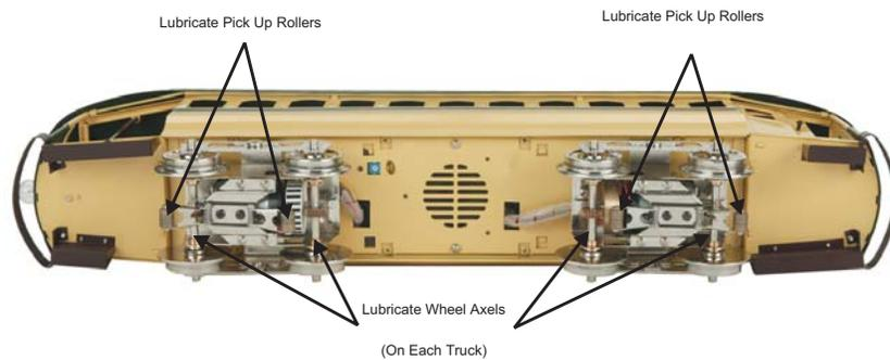
*Figure 1. Lubrication Points on the Trolley*
