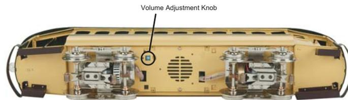
Figure 2: Manual Proto-Sound 2.0 Volume Adjustment
