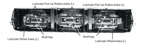
Figure 1. Lubrication Points on the Locomotive
