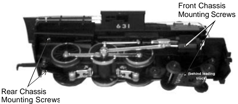
Figure 10: Removing The Boiler From The Chassis
