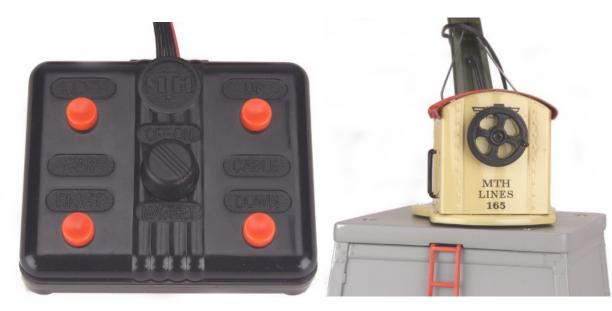
Caution: Only the "Right" and "Down" buttons or the "Left" and" "Up" buttons may be pressed simultaneously. Pressing any other two buttons at the same time will stall motor.
