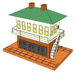
The Standard Gauge Switch Tower is illuminated with two internal 18-volt lamps and six knife switches capable of controlling up to 6 electrical accessories such as building lights, street lights and etc. Please refer to the following diagrams for illuminating the switch tower and suggestions for connecting your electrical accessories to get the greatest amount of enjoyment from your switch tower and standard gauge train layout.
