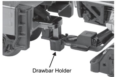
*Figure: Attaching the Plastic Drawbar Holder*
