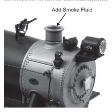
Running the engine without a primed smoke unit may cause damage
