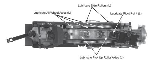
Figure: Lubricating the Locomotive
