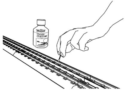
To clean the track, use RailKing® Track Cleaning Fluid or denatured (not rubbing) alcohol and a clean rag. Unplug the transformer and wipe the rails of the track, turning the rag frequently to ensure that you are using clean cloth on the rails. Thereafter, keep an eye on the track and clean it when it gets dirty to ensure good electrical contact and to lengthen the life of the tires.
