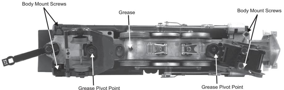
*Figure: Body Mount Screws and Grease Points on the K-4s Pacific*
