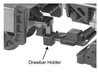
Figure: Attaching the Plastic Drawbar Holder
