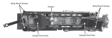
Figure: Body Mount Screws and Grease Points on the K-4s Pacific
