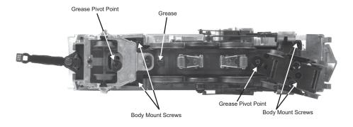
Figure: Body Mount Screws and Grease Points on the USRA Pacific
