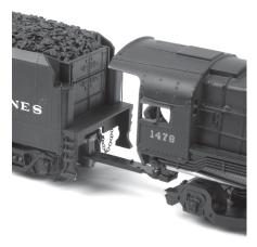
Figure: Connecting Locomotive to Tender
