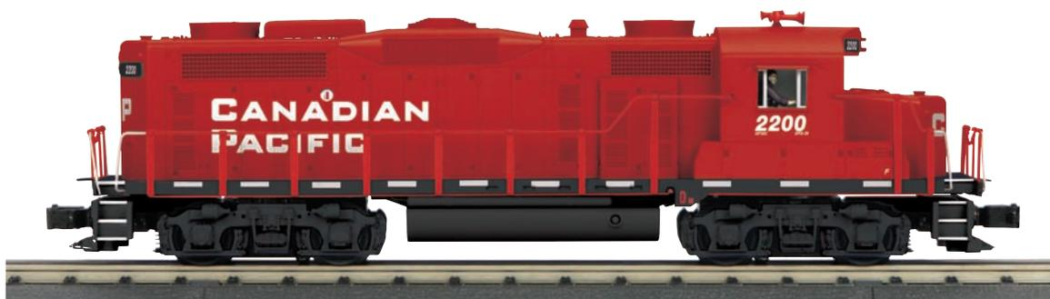
In the late '50s, railroads were looking for units with high-horsepower output. General Electric and Alco obliged by releasing units with 2,400 and 2,500-h.p. capability. General Motor's Electro-Motive Division, at first, was reluctant to chime in. They figured that turbocharging their 567 engine would drive up maintenance costs, and that was to be avoided. Yet, in 1959, EMD outshopped the GP20, a 16-cylinder, 2,000-h.p. road switcher, with its turbocharged 567D2 engine.
