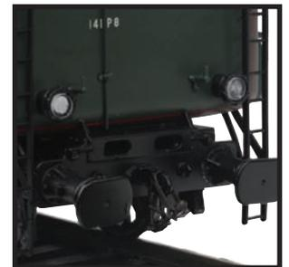
The 2-8-2 wheel arrangement — a 141 configuration in French parlance, which counts axles rather than wheels — was the most common steam locomotive configuration on French rails. Beginning in 1945 and lasting for 30 years, France's nationalized railroad was dominated by the American and Canadian-built SNCF 141R class with a total of 1,323 locomotives entering service.
