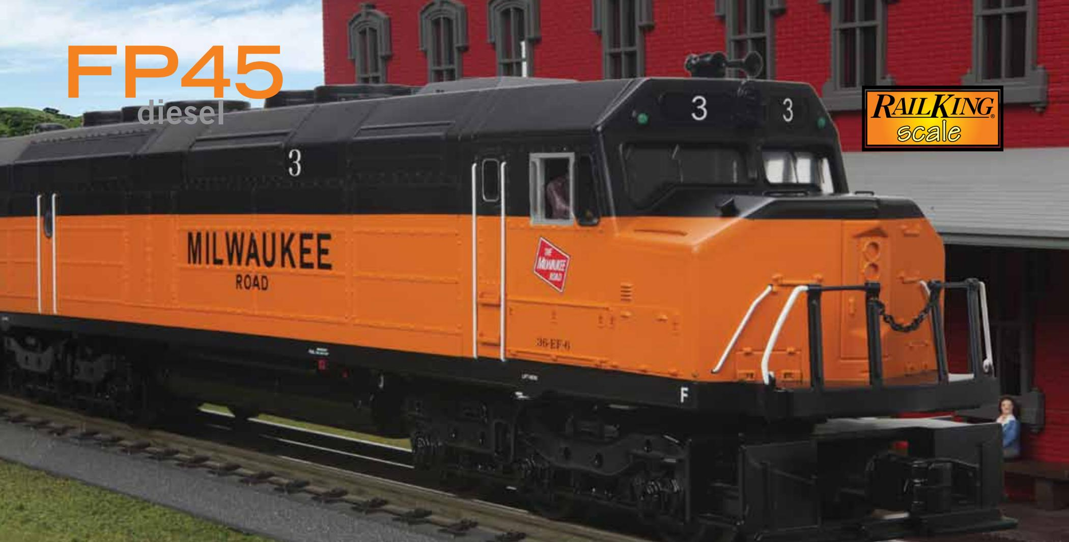
Designed in 1967 at the request of the Santa Fe, the FP45 was basically an SDP45 road switcher with a streamlined cab unit body. The "P" in FP45 indicated a passenger diesel with a steam generator for train heat. Having a sleeker, more aerodynamic look than a road switcher, the FP45 blended better with its passenger consists; the fully enclosed body also reduced wind resistance and allowed the crew to perform troubleshooting and minor maintenance on the road.
