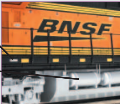
Die-Cast Air Tanks With Separately-Added Metal Pipes
